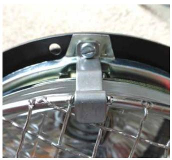
For another installation, such as on our #WP6 stainless headlamp, you must first separate the glass from the rim by removing the spring wire clips that hold the glass lens in place. Locate the shaped end of the three brackets, evenly spaced, over the edge of the glass between the glass and the rim, then refit the retaining springs. It's a bit fiddly and will require some patience or maybe an extra pair of hands.
