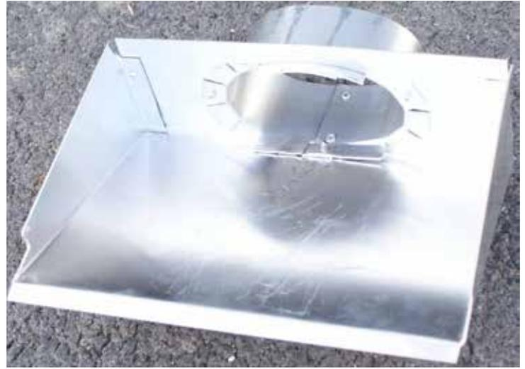
You can secure the plenum with rivets or even short self-tappers if you wish. If a top inlet is inappropriate for your installation, just redesign the plenum with a side inlet or simply turn the heater box on it's side.
