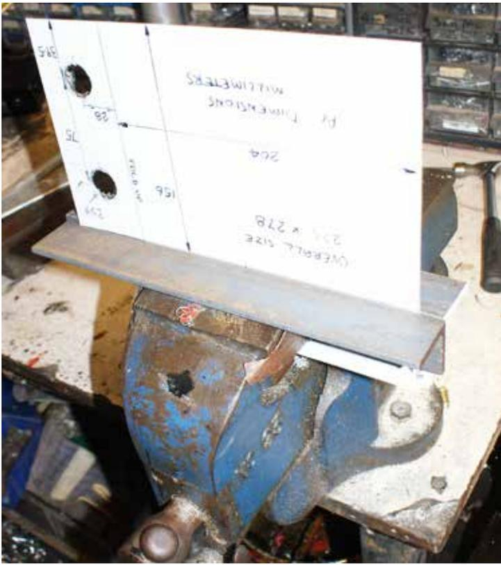
Picture 1 shows the two halves of the box 'Cleko'd' together. I've cut a large hole in one side as the air inlet to the matrix and I've mounted two bulkhead flanges on the opposite side as 'outlets'. There's plenty of room to mount more as you wish.
